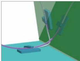
The harness follows the moving parts. The length of the harness is calculated automatically.
